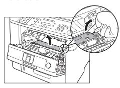
2 Slide and push the jammed paper into the machine until the front edge of jammed paper comes out.
